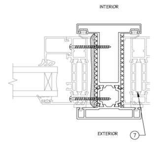
7. Install the window on the opposite side of the H-Mull using the same method.
