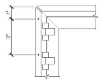
D. For Jambs, predrill ¼"dia holes every 12", starting 4" from both edges.
