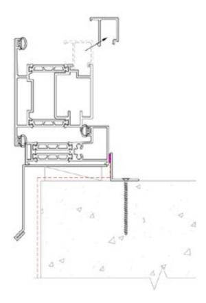
B. Apply a smear bead in the bottom cavity corners along the entire depth of the frame.
