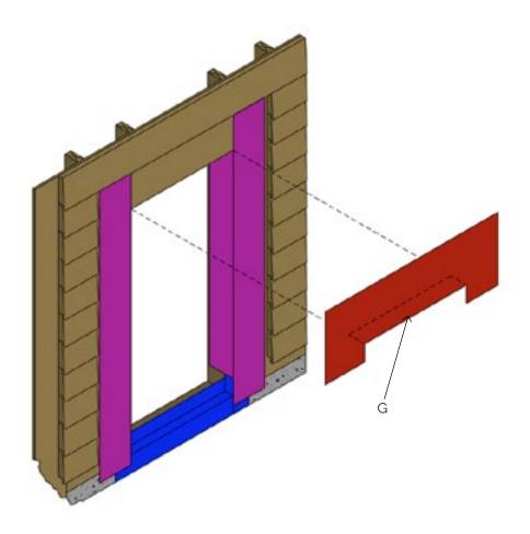
G. Apply a single ply of WRB/AB (VP100) to the head of the rough opening. Make a relief cut and tuck the WRB/AB (VP100) flap under the head of the opening.
